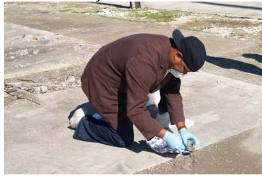
Figure 2. The sample collection procedure included use of protective equipment and documentation through chain of custody forms.
