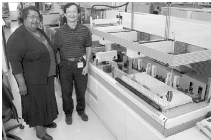
Beverly Campbell, manager of Laboratory Information Services (LIS), and Huy Nguyen, the LIS Systems Manager, stand with the FE500 instrument from TECAN. Instruments such as this have taken over much of what was done manually in the pathology lab. The FE500 works like its own assembly line and distribution system subdividing samples into various test tubes based on the number of tests ordered by doctors. The samples then move on to the various analyzers for testing.
